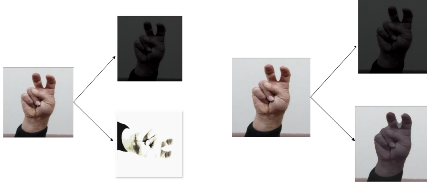
Fig. 3: global-global (left) and local-global augmentation (right), illustrated on an image from the ArASL dataset [19]. Local augmentation is applied to the RoI.
