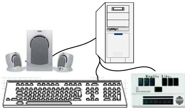
Figure 1.2b: Typical PC configuration for a blind person. It is composed of a vocal synthesizer, refreshable Braille device 1 and a keyboard (ASCII, Braille or specialized).
