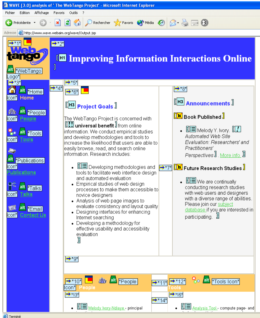
Figure 2.5: Evaluation report produced by WAVE. WAVE overlays guideline violations on the actual web page. It uses numerous icons to flag potential issues and also depicts the page reading order (arrows with numbers).
