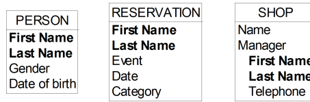
Figure 3.3: A simple schema with structural redundancies
