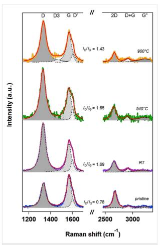
**Figure 4:** Raman spectra acquired on pristine, functionalized and thermally treated vCNTs. The spectrum at the top was recorded after heating the sample to  $T = 900\,^{\circ}\text{C}$ , which corresponds to a completely defluorinated sample. The spectra were normalized to the G-peak intensity.
