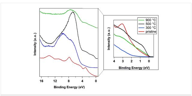
**Figure 3:** UPS spectra acquired with a photon energy of hv = 31 eV, the red line is the pristine vCNT sample, the blue is the functionalized, annealed (T = 300 °C) sample, the black and the green lines are related to samples heated at 500 and 900 °C, respectively.
