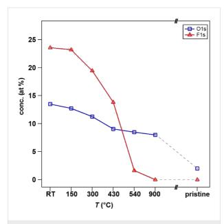
**Figure 2:** Atomic concentration of oxygen (blue squares) and fluorine (red triangles) calculated from XPS analysis as a function of heating temperature.
