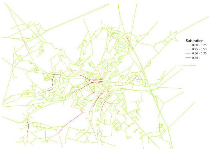
Fig. 8. Saturation of the Namur road network at 8:00 am - 100,000 agents, 360,000 trips, road network made of 25,000 nodes and 17,000 links.
