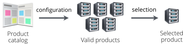
Fig. 11: The configuration phase and the selection phase for a catalogue of servers.
