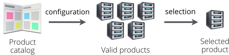
Fig. 11: The configuration phase and the selection phase for a catalogue of servers.
