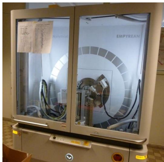
Figure 16. X-ray diffractometer of the Geological Survey (RBINS, Brussels) used for XRD analyses of powdered rocks.
