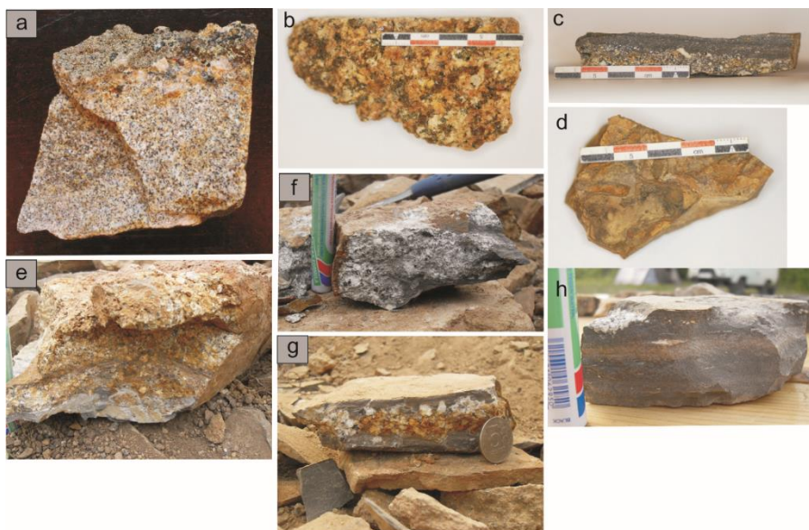
Supplementary Figure S5.5. Selected rock samples from Kulinda locality. The photographs show (a) a granite and (b) a biotite granite collected on top hill, (c) and (d) greywackes from trench 4, (e) and (f) breccia and brecciated sandstone from trench 3, (g) very coarse-grained sandstone and (h) mudstone from trench 3/3.
