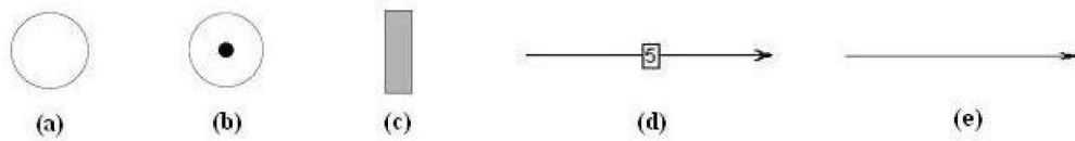
Fig. 7.1: (a) a place; (b) a place with a token; (c) a transition; (d) an arc labeled with the weight 5 ;(e) a unitary arc
