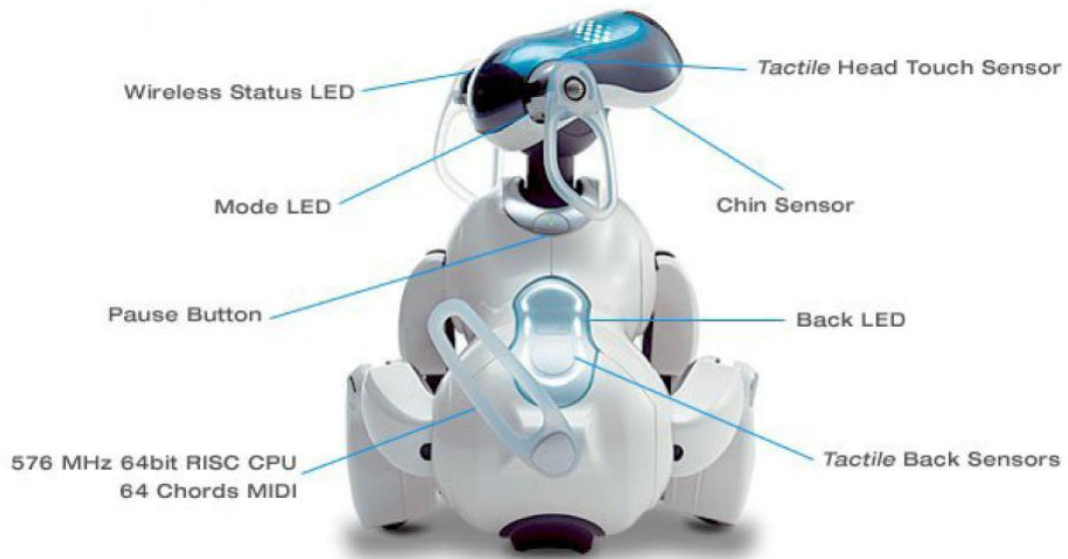
Fig. 4.2: Rear view of AIBO's ERS-7 hardware and peripherals [58], cited in [50]
