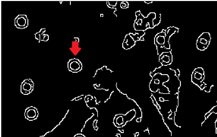
Figure 5.3: Zoom of the direct application of an edge detection filter. Pores appears clearly (red arrow). The image is too noisy, there is too much information.
