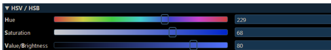
Figure 2.5: In HSV colour system, the hue can be selected independently from its saturation or brightness.
