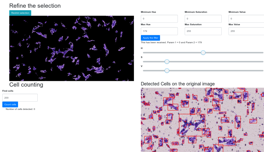
Figure A.19: Screen shot from the second page of the cell counting application with angular. The user can apply a second filter and launch the automatic enumeration.
