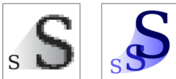
Figure 2.2: Comparison of a raster image (left) and a vector image (right). Vector images can be scaled up without losing quality [4].
