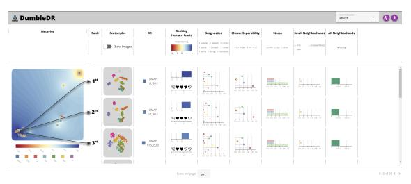
Fig. 9: Screen capture of the tool for ranking projections. The projections in the scatterplots column are ranked using Model 3. On the left of the ranking, a metamap shows similar projections close together and dissimilar ones far apart. The blue (resp. red) zone represent good (resp. bad) projections w.r.t. Model 3 scores. On the right of the ranking, the average number of hearts given by participants is shown, as well as individual quality metrics values.
