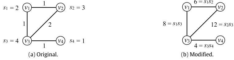
Fig. 2. Strength-biased RW. (a) An original undirected network, whose weighted adjacency matrix is given by A . (b) The modified undirected network, whose weighted adjacency matrix is given by A' . The numbers attached to the edges represent the edge weight. We set \alpha = 1 .
