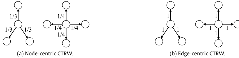
Fig. 3. Schematic of two types of continuous-time random walks (CTRWs) on networks: (a) a node-centric CTRW and (b) an edge-centric CTRW. In each case, a walker is visiting either a degree-3 node or a degree-4 node in a network, which we assume is unweighted for simplicity. We show the transition rates for each edge. In panel (a), the walker travels at a unit rate and moves to one of its out-neighbors with equal probability for each choice. Therefore, the transition rate for each edge is the reciprocal of the out-degree of the node that the walker is visiting. In panel (b), however, the transition rate on each edge is equal to 1. Therefore, on average, a walker visiting the node with out-degree 4 leaves the node earlier than a walker visiting the node with out-degree 3.
