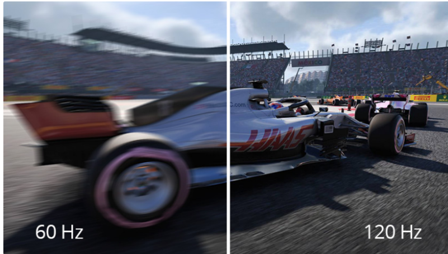
Figure 2.2: Example of refresh rate effect on moving cars, from 60 Hz to 120 Hz. Higher the refresh rate is, smoother the picture will be. Picture found on www.coolblue.be
