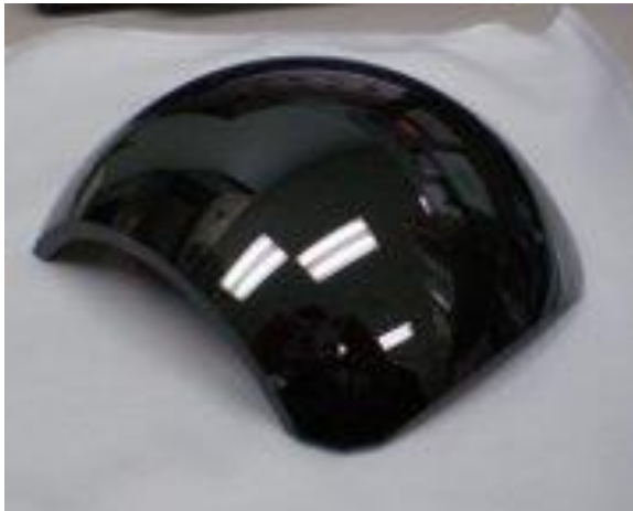
Figure 1.7 Dome coated with DLC for optical and tribological purposes. 6
