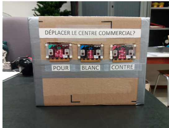
Figure 6.6: Vote counter displaying the aggregated results from the voting boxes developed by the children.
