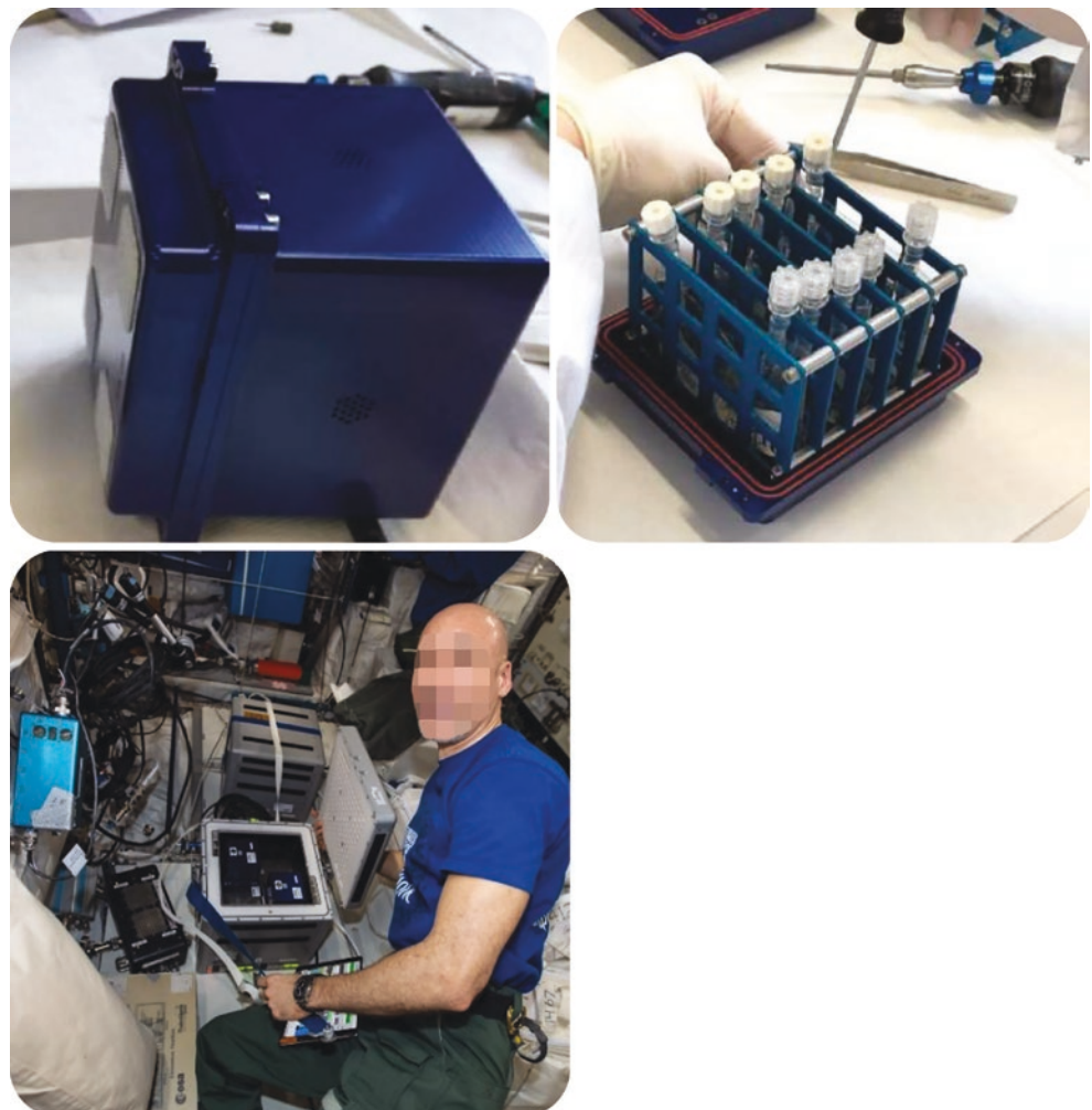
Fig. 10.20 View of Rob1 hardware used to culture hydrated A. vaga individuals onboard of ISS (December 2019). Top left: Rob1 hardware after its assembly at the launch site at Kennedy Space Center. Rob1 hardware is a passive hardware containing five culture bags containing hydrated specimens of A. vaga . Hardware enables gas exchanges between rotifer cultures and the outside through a permeable membrane. Top right: View of the culture bags assembled inside Rob1 hardware. Culture bags, loaded with 10,000 A. vaga individuals each, are made of Teflon and ensure an optimal gas exchange between the culture medium and the outside. Bags are waterproof and avoid any leakage of the medium (composed of mineral water and sterile lettuce juice) or rotifers. Reprinted with permission of Marc Guillaume. Bottom left: View of ESA astronaut Luca Parmitano loading two Rob1 hardware on KUBIK. KUBIK is a small incubator, temperature-controlled, with removable inserts designed for self-contained microgravity experiments. (Reprinted with permission of NASA)
