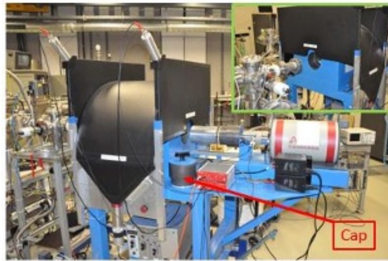
Figure 1: General view of the low background \gamma -ray detector at the LARN. One can see three plastic scintillators (in black) surrounding the lead castle (in blue). The whole system (i.e. HPGe - lead castle - scintillators) is mounted on a sliding tray which enables to move it close to or away from the end of the beam line.
