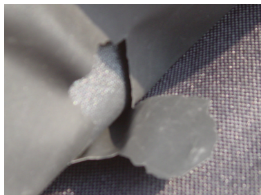
Figure 4.3: A too fragile pocket separator
