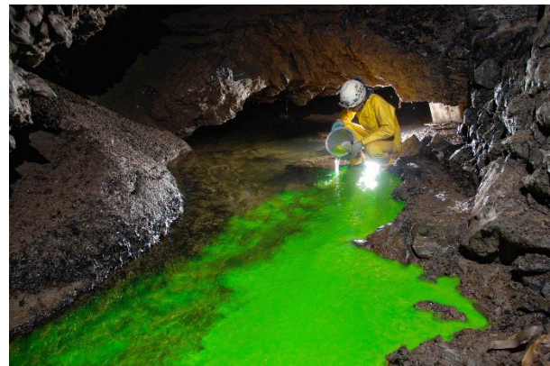
Figure 2. Uranine injection in the Lorette cave river during low water conditions.
