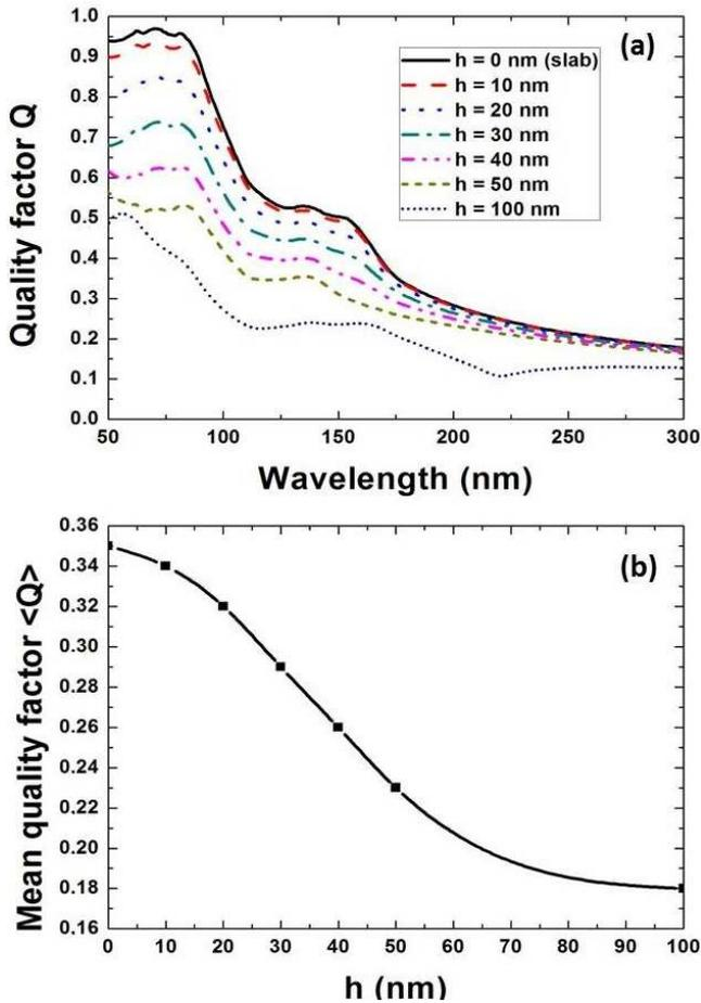
FIG. 5: (Color online). (a) Quality factor  $Q$  of the Fabry-Perot cavity formed by the flat polyethylene slab and the patterned polyethylene slab.  $Q$  is given against the wavelength for various cone heights. (b) Mean value (integration over wavelength) of the quality factor of the cavity described above. Both slabs are separated by water.
