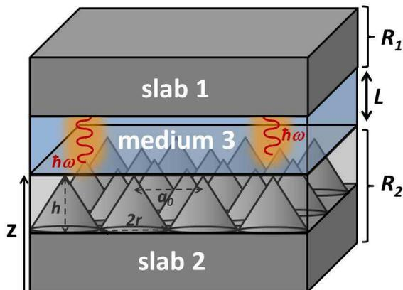
FIG. 1: (Color online). Bodies 1 and 2 interacting *via* an intervening medium 3. The two bodies are separated by a distance  $L$ .  $R_1$  ( $R_2$ ) is the Fresnel reflection coefficient of slab 1 (slab 2). The surface of body 2 is nanopatterned with corrugations that are described by a graded effective medium.
