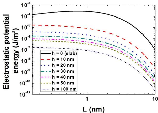
FIG. 10: (Color online) Electrostatic potential energy between PE slabs as a function of cones height. Note the orders of magnitude on the Y-axis in comparison with Fig. 4.
