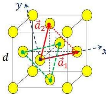
Figure 5. Orientation of two basis vectors of the unit cell (parallel to the chitin layer) in the FCC lattice. Two reticular planes are highlighted in green and red. The norm  $a$  of vectors  $\vec{a}_1$  and  $\vec{a}_2$  is equal to the distance between two neighboring perforation centers. (colors available online)
