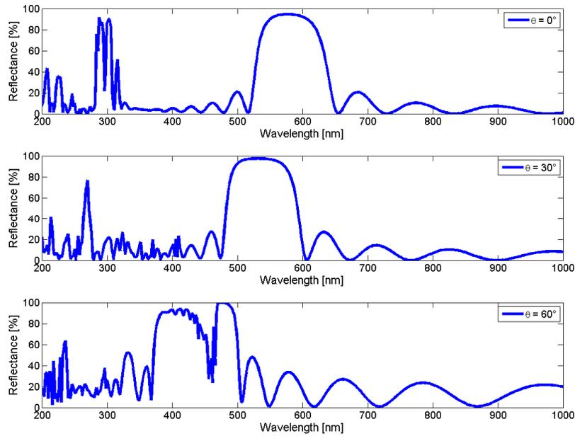
Figure 8. Reflectance spectra calculated for the (111) direction of the photonic crystal at incidence angles  $\theta$  equal to  $0^\circ$ ,  $30^\circ$  and  $60^\circ$  (from top graph to bottom graph).
