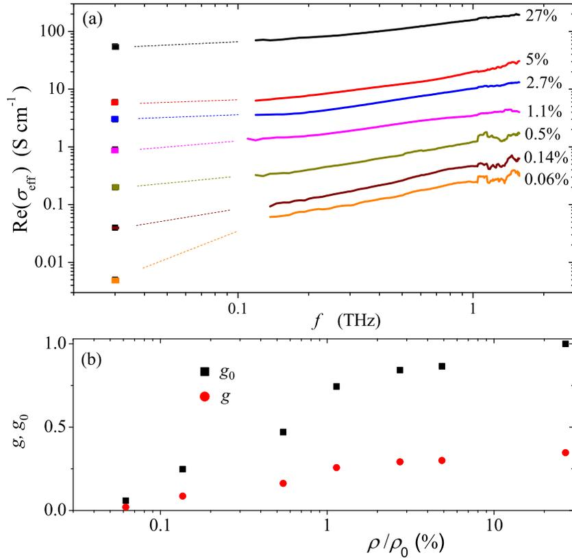
Figure 4: (a) Frequency dependence of  $\text{Re}(\sigma_{\text{eff}})$  for the CNT/INT film at different CNT volume fractions  $\rho/\rho_0 \in \{0.06, 0.14, 0.5, 1.1, 2.7, 5\}\%$ ;  $\rho$  is a density of CNTs;  $\rho_0 = 2.2 \text{ g/cm}^3$  is the density of graphite; for pure CNT film  $\rho/\rho_0 = 27\%$ ; (b) The parameters  $g(30\text{GHz}, 1\text{THz})$  and  $g_0(30\text{GHz}, 1\text{THz})$  calculated from data presented in (a) versus  $\rho/\rho_0$ .
