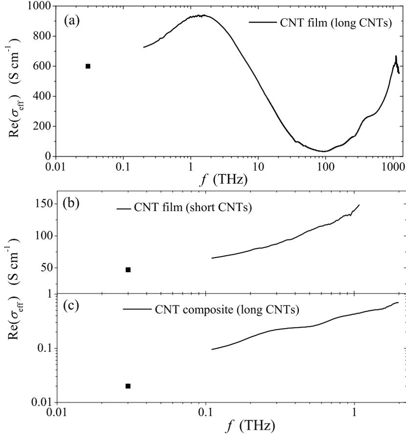
Figure 3: Frequency dependence of  $\text{Re}(\sigma_{\text{eff}})$  for the film comprising (a) long, and (b) short CNTs, and (c) for CNT-polymer composite containing 1 wt% of long CNTs. Black square symbols indicate the conductivity of the samples at 30 GHz.
