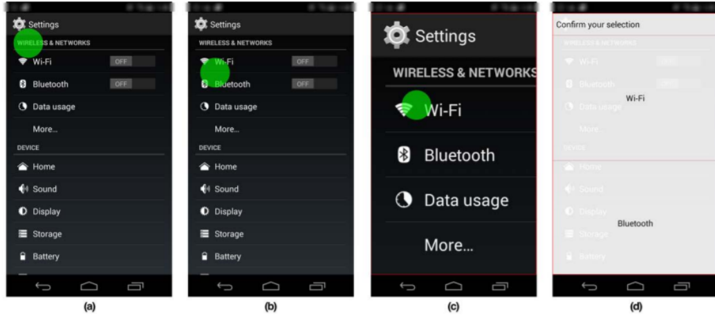
Figure 3.25: Touch Guard: (a) touch without ambiguity, (b) touch with ambiguity (on multiple targets), (c) magnification disambiguation, (d) targets list mode disambiguation (taken from (Zhong et al., 2015))
