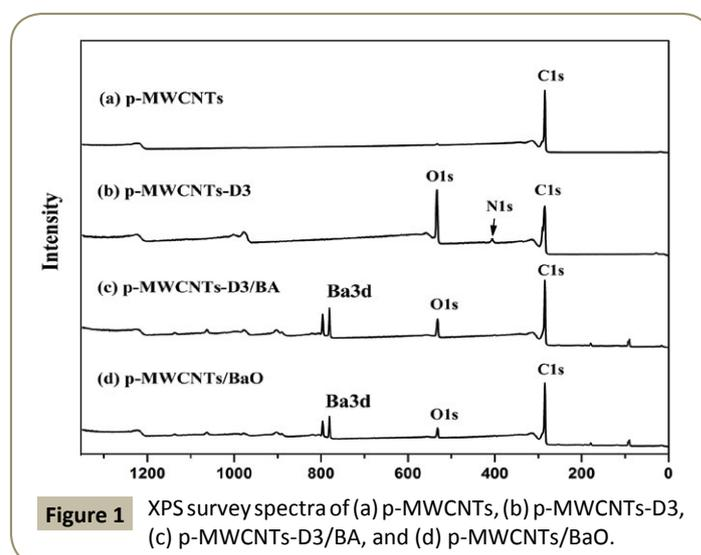
**Figure 1** XPS survey spectra of (a) p-MWCNTs, (b) p-MWCNTs-D3, (c) p-MWCNTs-D3/BA, and (d) p-MWCNTs/BaO.
