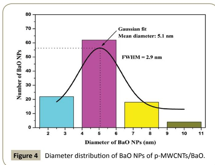
Figure 4 Diameter distribution of BaO NPs of p-MWCNTs/BaO.
