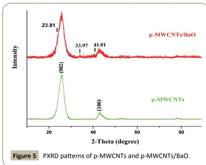
Figure 5 PXRD patterns of p-MWCNTs and p-MWCNTs/BaO.
