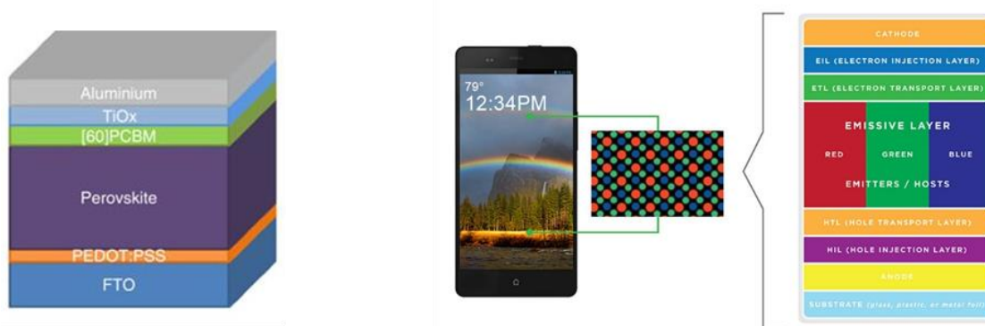
Figure 1 - Example of structures found in hybrid organic/inorganic devices. Left: Perovskite solar cell [9] ; Right: OLED for display application [Source: https://oled.com/oleds/ ].
