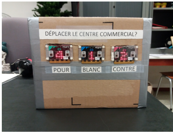
Figure 5: Cardboard box holding three micro:bits, one per voting option ( in favor, blank, against ).
