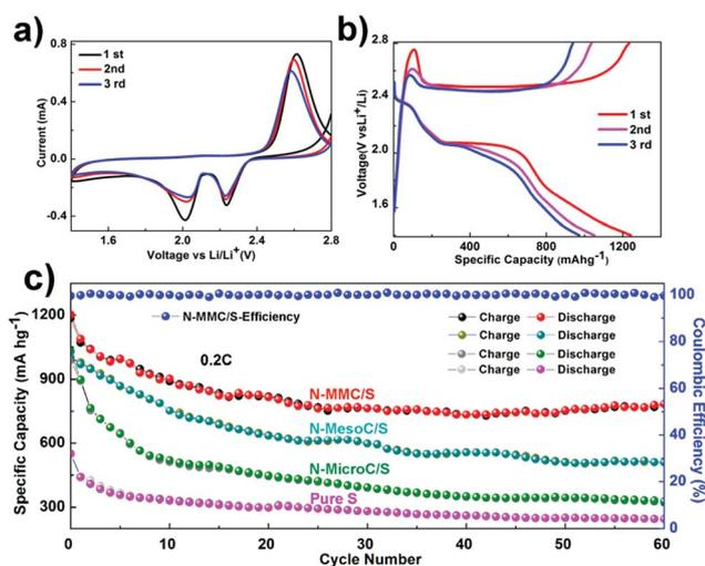
Fig. 4 (a) CV curves of N-MMC/S electrode at a sweep rate of  $0.2 \text{ mV s}^{-1}$  in the potential range from 1.40 V to 2.80 V vs.  $Li/Li^+$ . (b) The discharge/charge profiles of N-MMC/S electrode cycled at 0.2C. (c) The cycling performances at 0.2C.
