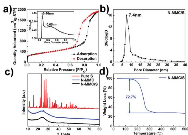
Fig. 2 (a)  $\text{N}_2$  adsorption–desorption isotherm plot of N-MMC, the inset is the corresponding micropore size distribution of N-MMC. (b) Mesopore size distribution of N-MMC. (c) XRD patterns of N-MMC, N-MMC/S and pure sulfur. (d) TG curves of N-MMC/S.
