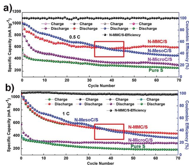
Fig. 5 The cycling performances of N-MMC/S, N-MesoC/S, N-MicroC/S and pristine S electrodes at different current densities of (a) 0.5C and (b) 1C.
