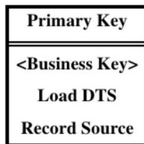
FIGURE 11 – Structure d’un hub. (GRAZIANO 2011b)
