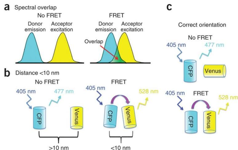
**Figure 13** – Parameters influencing FRET efficiency. Cyan fluorescent protein (CFP) is donor and Venus is acceptor. a: Spectral overlap of the donor and the acceptor spectra is needed. b: Separation of the donor and the acceptor smaller than 10 nm is essential. c: Correct orientation of the acceptor towards the donor must be respected. Taken from Northwestern University [48].
