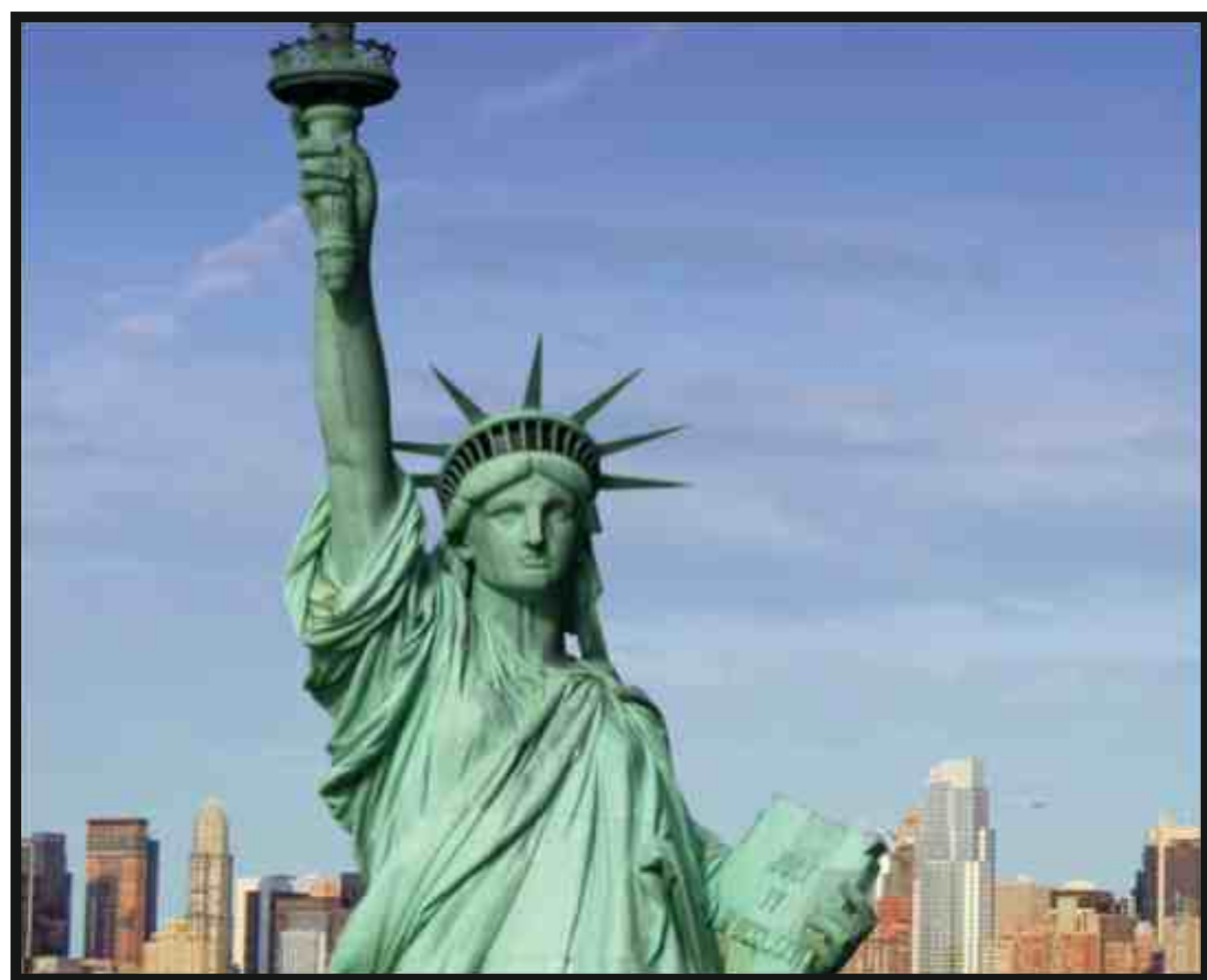
Figure 4 - Cu sulfates and carbonates (weathering) give the characteristic green color to the Statue of Liberty.
