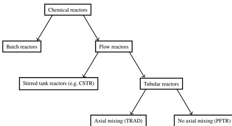
Figure 1.2 – Different types of chemical reactors.
