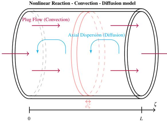
Figure 1.3 – Profile view of a plug-flow tubular reactor with axial dispersion actuated by a surrounding heat exchanger.
