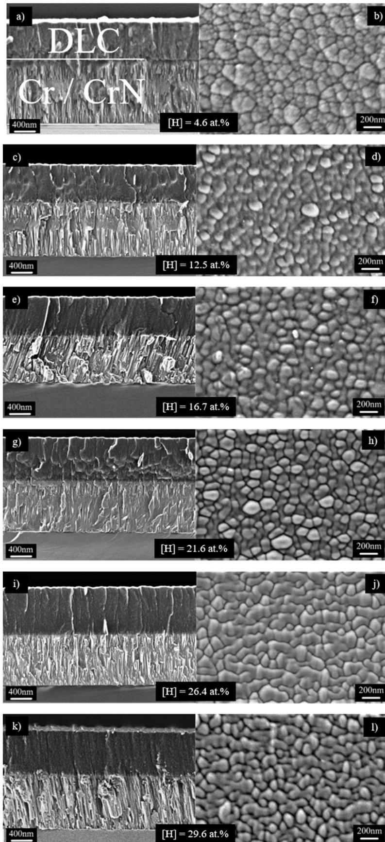
Fig. 5. Cross-sectional (left) and conventional (right) SEM micrographs for the samples synthesised in various Ar:CH<sub>4</sub> gas mixtures (see Table 1).
