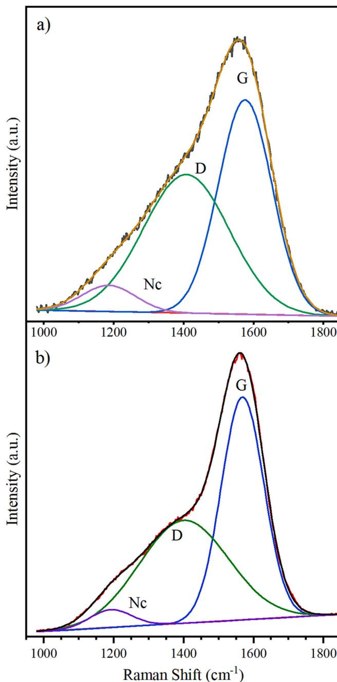
Fig. 7. Raman spectra of the DLC films deposited with a) 1.25 % and b) 10 % CH<sub>4</sub> in the plasma.
