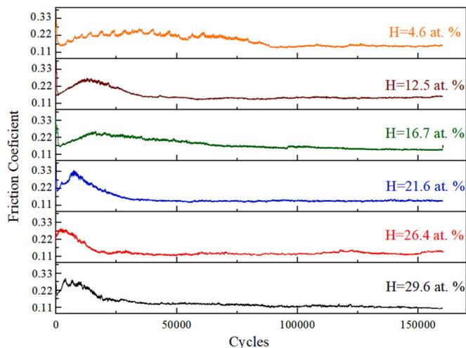
**Fig. 9.** Coefficient of friction during the pin-on-disk tests.
