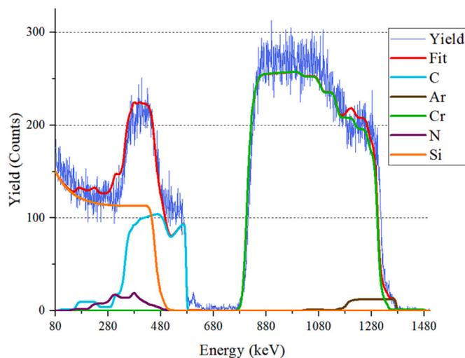
**Fig. 2.** RBS spectrum acquired at 4.3 MeV at  $135^\circ$  for the sample deposited with 1.25 % of  $[\text{CH}_4]/[\text{Ar} + \text{CH}_4]$  ratio in the Ar:CH<sub>4</sub> mixture. The experimental spectrum is shown in light purple, while the red curve indicates the fitted spectrum. The latter comes from the contributions of the different elements contained in the sample: the silicon backing (orange), chromium (green), nitrogen (dark purple), carbon (light blue) and argon (brown).
