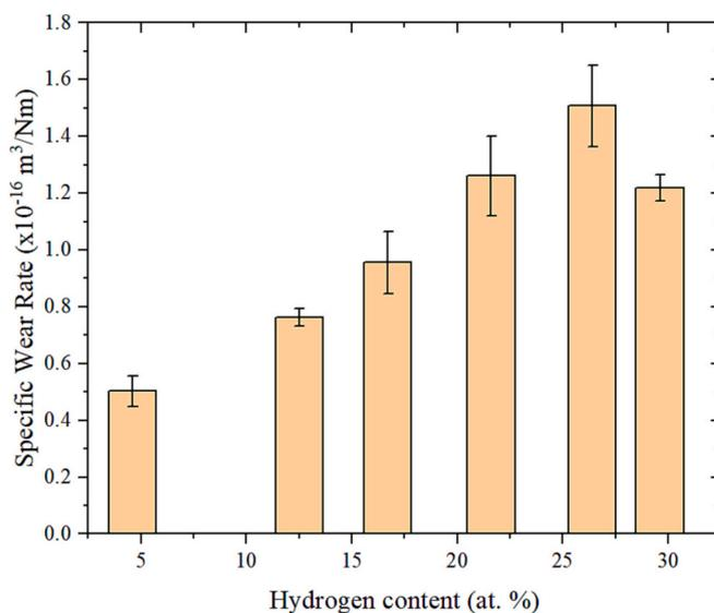
Fig. 13. Specific wear rates of the DLC films as a function of the hydrogen content.
