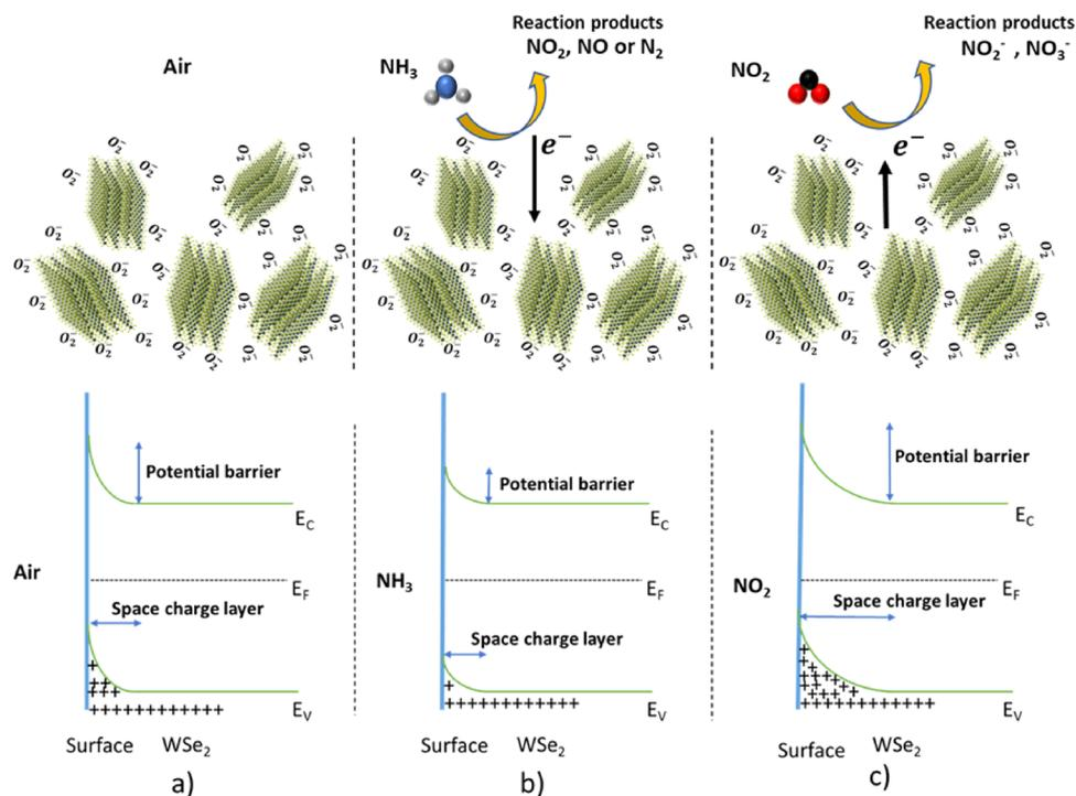
**Figure 14.** Schematic sketch of NH<sub>3</sub> and NO<sub>2</sub> gas sensing mechanisms and associated energy band diagrams for 2H WSe<sub>2</sub> (a) in air, (b) in the presence of NH<sub>3</sub>, (c) in the presence of NO<sub>2</sub>, where E<sub>C</sub>, E<sub>F</sub>, and E<sub>V</sub>, correspond to the conduction band, Fermi level, and valence band.
