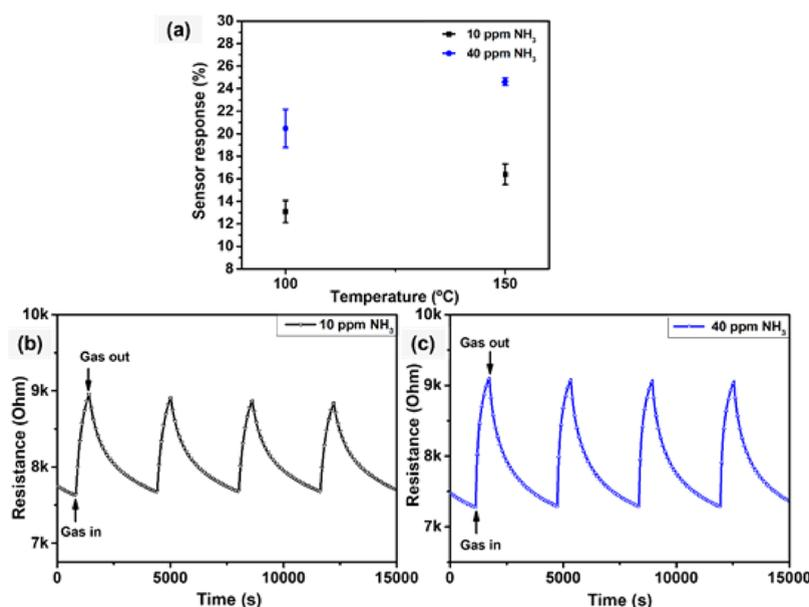
**Figure 9.** (a) WSe<sub>2</sub> sensor response as a function of temperature toward NH<sub>3</sub> gas, (b) film resistance change as a function of time toward (b) 10 ppm of NH<sub>3</sub> and (c) 40 ppm of NH<sub>3</sub>, at 150 °C.
