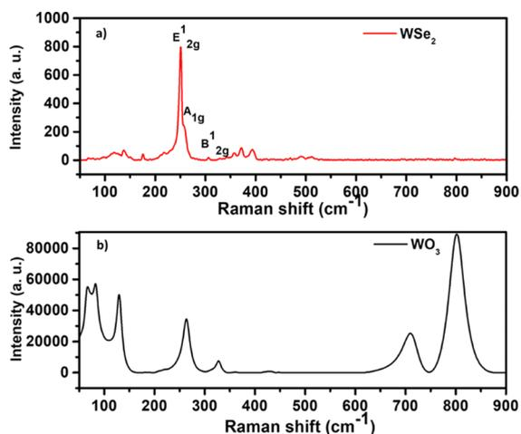
**Figure 4.** Raman spectra of (a) as-grown WSe<sub>2</sub> nanoflowered film and (b) WO<sub>3</sub> nanowires.
