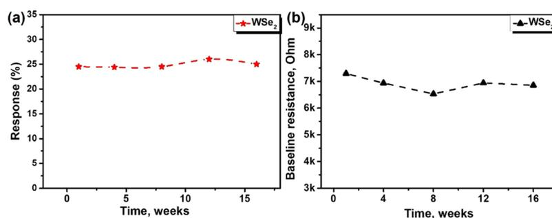
**Figure 13.** Long-term stability study. (a) Stability study for the WSe<sub>2</sub> sensor toward NH<sub>3</sub> gas over time, (b) evolution of the baseline resistance with time.
