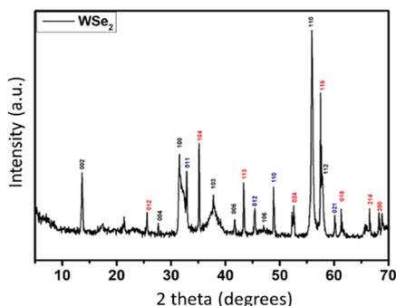
**Figure 5.** XRD diffractogram of as-grown WSe<sub>2</sub> nanoflowered film on alumina substrates with screen-printed platinum electrodes. Peaks whose crystal planes appear in red correspond to the alumina substrate on which the WSe<sub>2</sub> films were grown.
