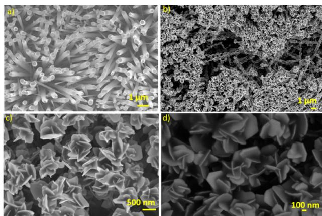
**Figure 2.** SEM and FESEM images depicting the growth of vertically aligned (a) WO<sub>3</sub> nanowires, (b) WSe<sub>2</sub> nanoplatelets, and (c,d) WSe<sub>2</sub> nanoflowers.
