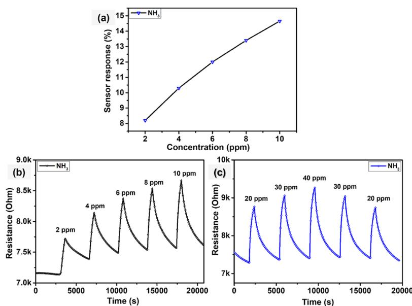
**Figure 10.** (a)  $\text{WSe}_2$  sensor response as a function of  $\text{NH}_3$  concentrations, (b,c) film resistance change as a function of time toward different concentrations of  $\text{NH}_3$  at  $150^\circ\text{C}$ .
