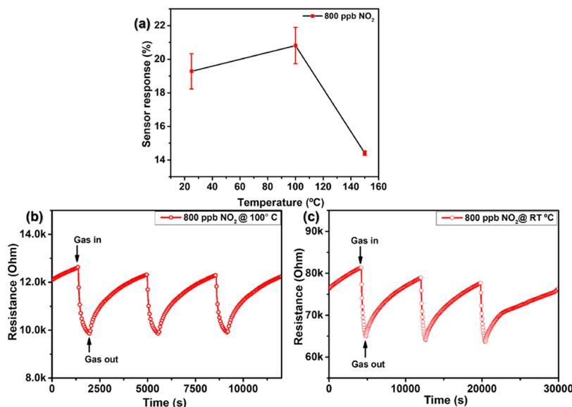
Figure 7. (a) Typical  $\text{WSe}_2$  sensor response as a function of temperature toward  $\text{NO}_2$  gas, (b) film resistance change as a function of time, toward 800 ppb of  $\text{NO}_2$  at 100 °C, and (c) film resistance change as a function of time toward 800 ppb of  $\text{NO}_2$  at 25 °C.
