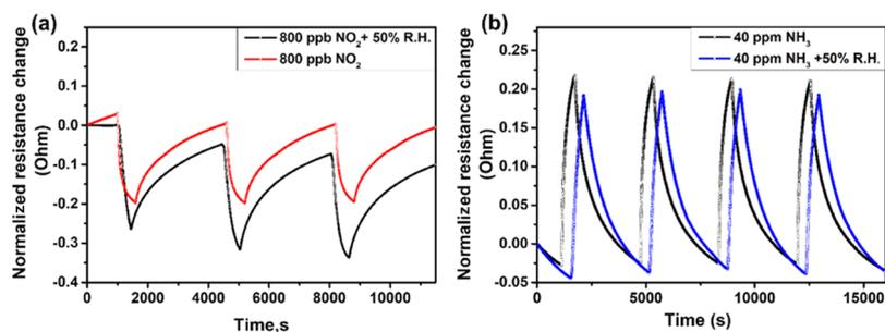
**Figure 11.** Dry and relative humidity cross-sensitivity to (a)  $0.8\text{ ppm NO}_2$  at  $100^\circ\text{C}$  and (b)  $40\text{ ppm NH}_3$  at  $150^\circ\text{C}$ .
