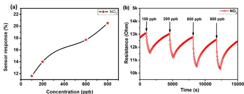
**Figure 8.** (a) WSe<sub>2</sub> sensor response as a function of different NO<sub>2</sub> concentrations and (b) film resistance change as a function of time, toward different NO<sub>2</sub> concentrations, at 100 °C.
