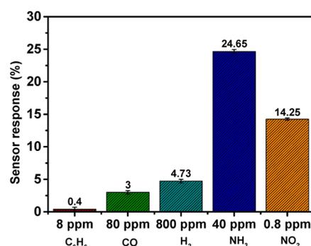
Figure 12. WSe<sub>2</sub> nanoflower sensor response based on exposure to 8 ppm C<sub>6</sub>H<sub>6</sub>, 80 ppm CO, 800 ppm H<sub>2</sub>, 40 ppm NH<sub>3</sub>, and 0.8 ppm NO<sub>2</sub> gas at an operating temperature of 150 °C.
