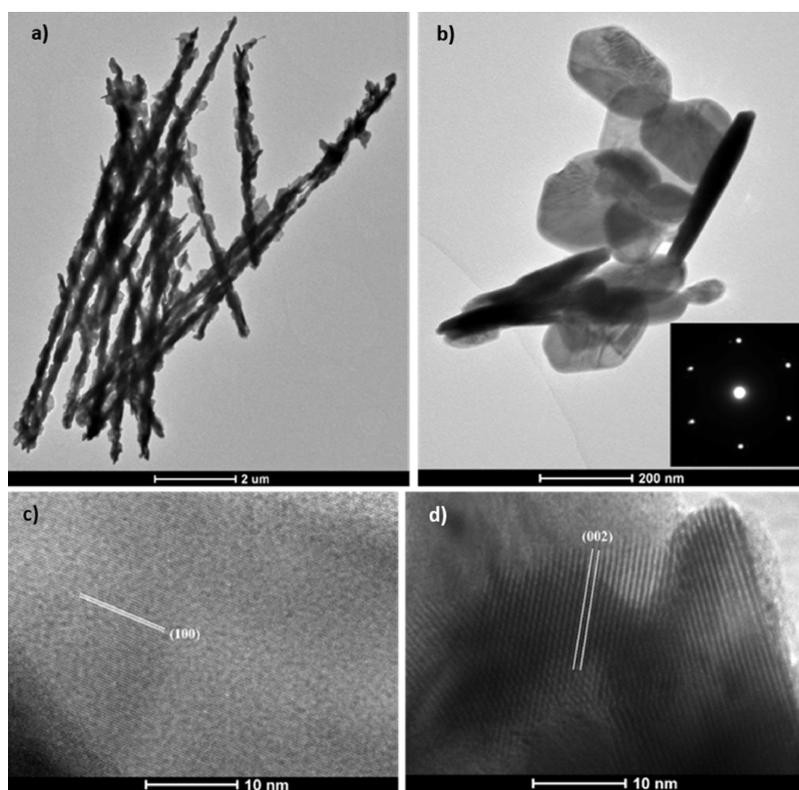
**Figure 3.** Low-magnification TEM images of (a) WSe<sub>2</sub> nanowires and (b) WSe<sub>2</sub> nanoflower petals with an inset of the SAED pattern along the [100] axis and high-resolution images of (c) a petal showing the (100) crystal planes and (d) layered structures of WSe<sub>2</sub> nanoplatelets composed of the petals with the (002) interlayer spacing.
