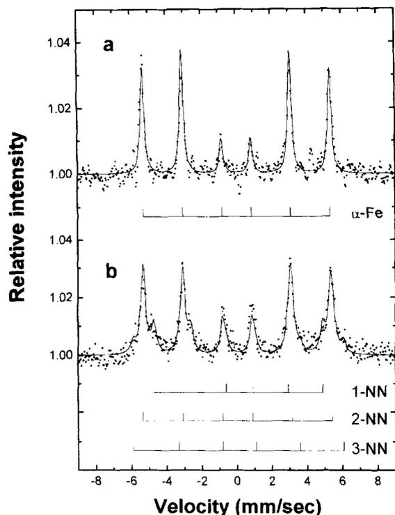
Fig. 2. CEMS spectra taken at room temperature on iron implanted with 100 keV  $^{15}\text{N}_2^+$  to a dose of  $1.3 \times 10^{17}$  ions  $\text{cm}^{-2}$ . The temperature during implantation was 120°C for (a) and 20°C for (b).
