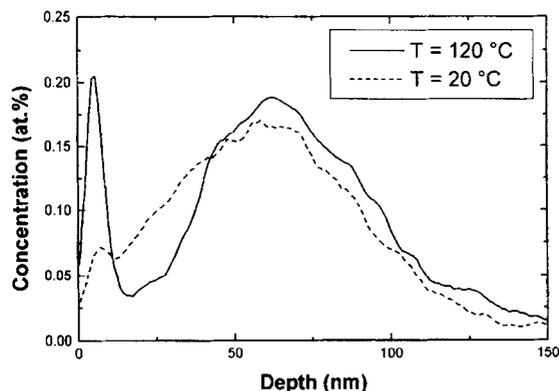
Fig. 1. Nitrogen depth profiles for pure iron implanted with 100 keV  $^{15}\text{N}_2^+$  to a dose of  $1.3 \times 10^{17}$  ions  $\text{cm}^{-2}$ . The full line corresponds to the specimen implanted at 120°C and the dotted line to the specimen implanted at room temperature.
