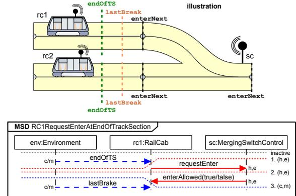
Figure 2. The MSD RC1RequestEnterAtEndOfTrackSection from the RailCab example
