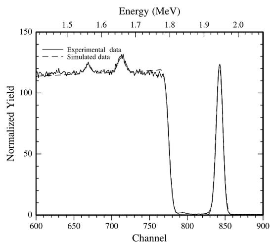
Fig. 1. A forward scattering spectrum of a  $\text{ZrO}_2/\text{Al}_2\text{O}_3/\text{Si}$  (2 nm/1 nm/ $\infty$ ) layer obtained with a 2 MeV  $\text{He}^+$  beam. Sample normal is tilted by  $45^\circ$  and the exit angle is  $6^\circ$ . The accumulated  $\text{He}^+$  dose was 100  $\mu\text{C}$ .
