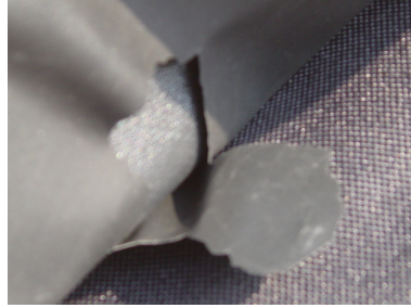
Figure 4.3: A too fragile pocket separator
